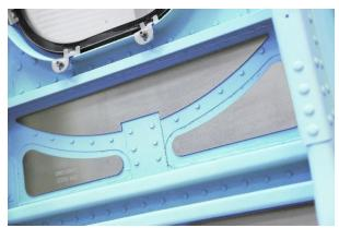
SMACSONIC® damping products are used on lightweight structures including fuselages, fairings, cabinets, crew rest compartments and monuments. As a complementary material to SMACSONIC®, SMAC will exhibit on Aircraft Interiors Expo SMACBARRIER®, a dense and thin acoustic barrier designed to offer flexibility even at low temperatures. SMACBARRIER® can be integrated in thermal blankets or on its own behind trim panels.
